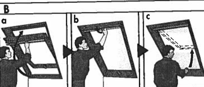
**ENGLISH:** Connecting springs to fittings: Close window using control bar (a, b). Then open window using handle on bottom of sash (c). Push sash outwards, ensuring that fittings and springs on both sides automatically connect (d).
