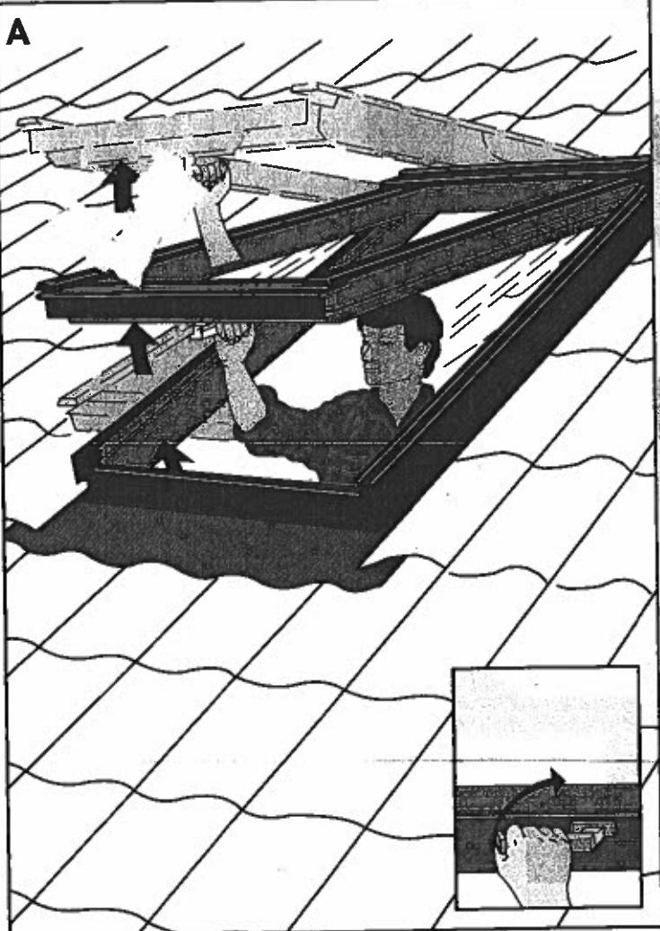
**ENGLISH:** Open window by turning handle to vertical position. The sash should be able to remain in any open position. If not, check that fittings and springs connect on both sides (see section B). If the sash still cannot remain in any open position, adjust springs (see section C).
